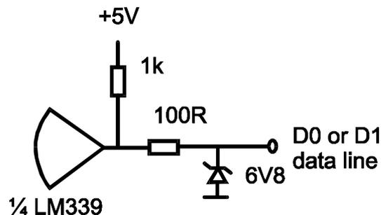
Wiegand output circuit schematic
