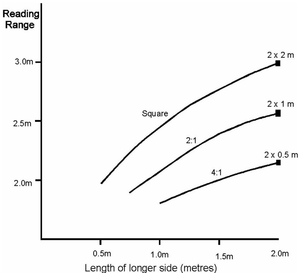
**Figure 3 - Graph of reading range against loop size (single turn)**
