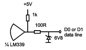
Wiegand output circuit schematic Figure 5
