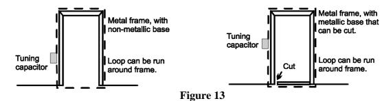
If there is a closed loop where you would like to place the aerial, it may be possible to break it without doing any damage. (**Before you make a cut, you must make sure that it won't affect structural integrity.**) If there is just a metal strip across the base, it may be possible to shorten one end by a small amount, breaking the closed
