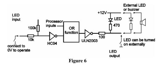
External LEDs and buzzer can also be used. These will totally mimic the state of the internal LEDs and buzzer. Connect an external LED <u>and its series resistor</u> between the LED output terminal and +12V. External buzzers can also be connected between the terminal and +12V, but don't need a series resistor. You must ensure that the LED or buzzer that you use is suitable and that it is properly decoupled to minimise effect on power lines.
