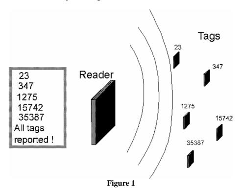
The tags are coded with a 64 bit identity number, although many applications will only use 32 of these 64 bits. The number of bits that are read, and the way those bits are formatted in the output from the reader, are determined by the reader's software. The reader's software has been designed in such a way that it can easily be configured to meet many common requirements.
