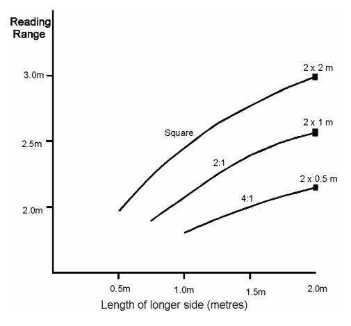
Figure 3 - Graph of reading range against loop size (single turn)
