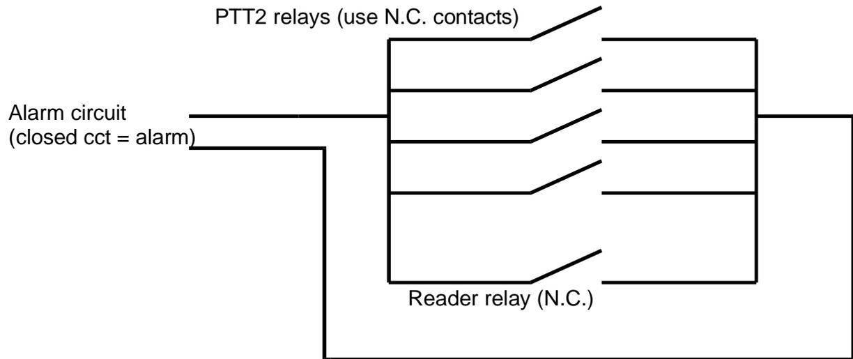
**(b) Parallel connected, using normally closed contacts that open in correct operation**
